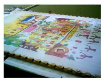
Figure 1 Coloring process, the fabric being mounted into a portable frame.
