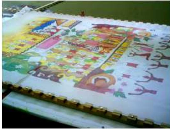
**Figure 1** Coloring process, the fabric being mounted into a portable frame.
