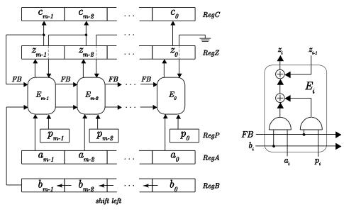
Figure 1 Serial PB Multiplier *GF*(2*m*).
