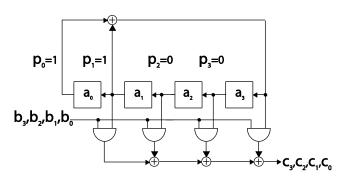
**Figure 4** DB serial multiplier with constant P(x).
