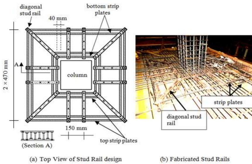
**Figure 10** Integrated stud rail of specimen 3.
