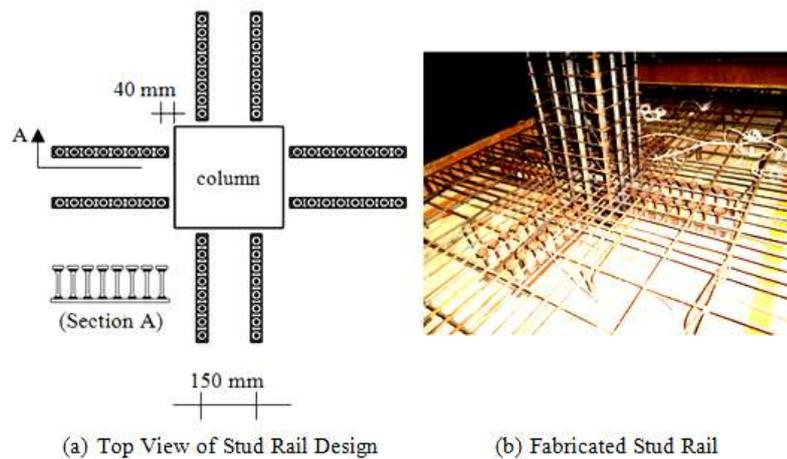
**Figure 8** Standard orthogonal stud rail configuration of specimen 1.
