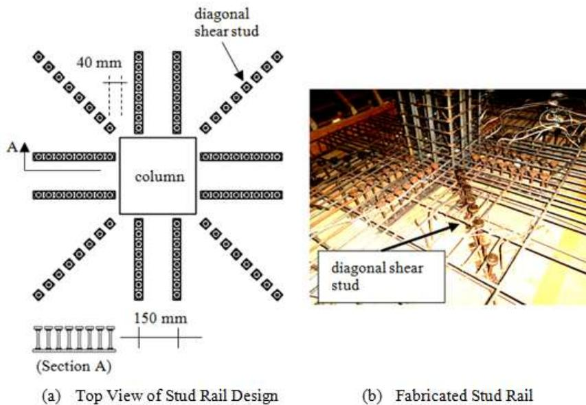
**Figure 11** Standard plus diagonal stud rail of specimen 4.
