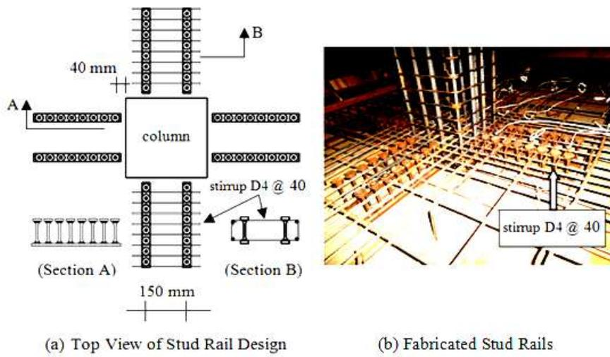
**Figure 9** Stud rail and stirrup configuration of specimen 2.
