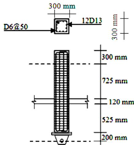
Figure 5 Column reinforcement.
