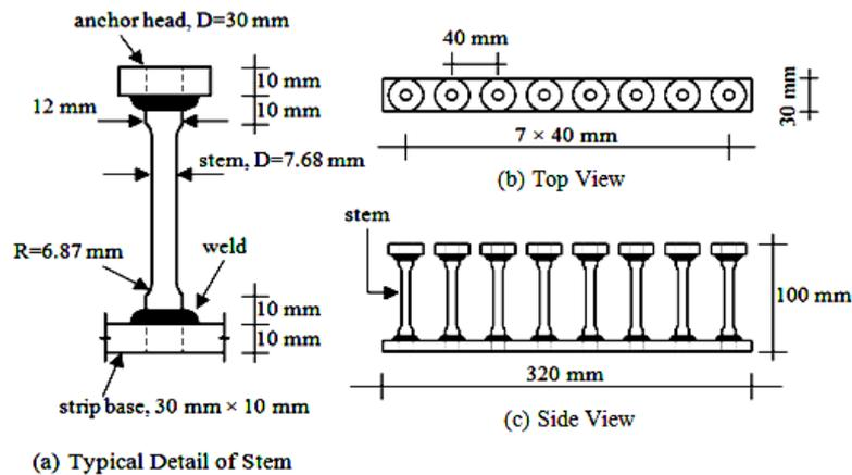
Figure 6 Bottom-up stud rail for specimens 1, 2, and 4 [11].
