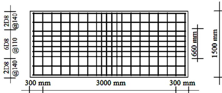
**Figure 4** Plan of slab bottom reinforcement.
