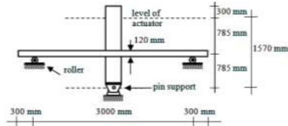
**Figure 13** Structural system of the specimens.
