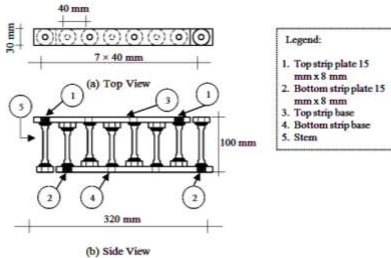
**Figure 7** Bottom-up and top-down stud rail of specimen 3 [11].
