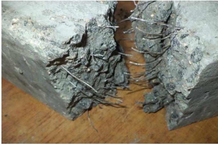
Figure 13 Effective fibre bridging showing pullout resistance
