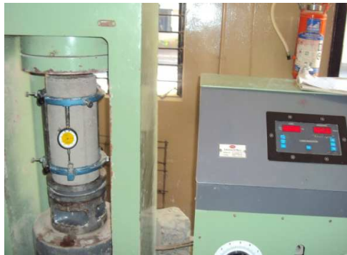
Figure 4 Test setup for Young's Modulus of concrete.
