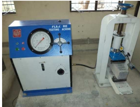
Figure 5 Test setup for flexural testing.
