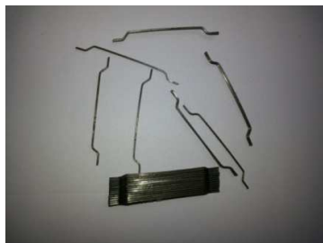
Figure 3 Snapshot of glued steel fibres (GSF) used in this study.
