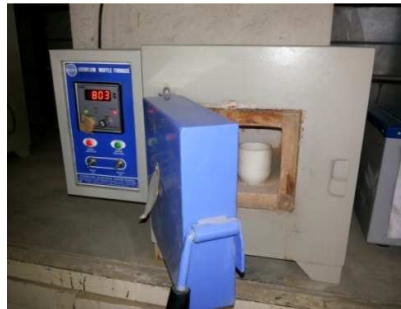
Figure 1 Rice husk ash sintered at 800°C in Muffle furnace.
