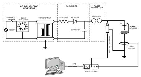
Figure 1 Schematic diagram of experimental system.
