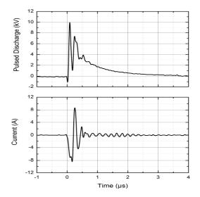
Figure 2 Waveform of the pulsed high voltage and current.
