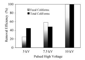
Figure 4 Effect of pulsed high voltage on removal efficiency of microorganisms.
