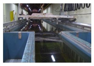
Figure 2 Towing tank facility
