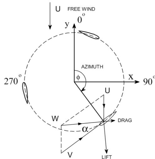
**Figure 1** Illustration of Darrieus concept.
