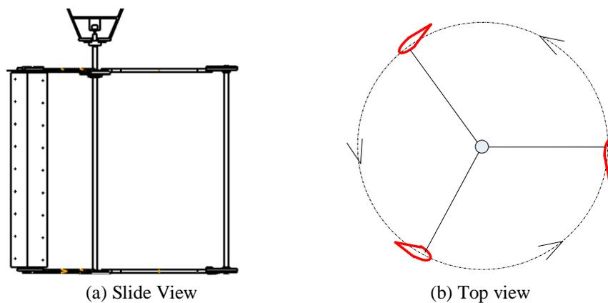
**Figure 3** Three straight blade vertical axis turbine.
