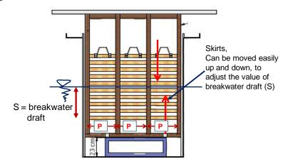
Figure 5 Sketch of draft adjustment (front view).
