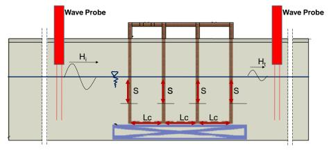
Figure 7 Sketch of PSB model (side view)
