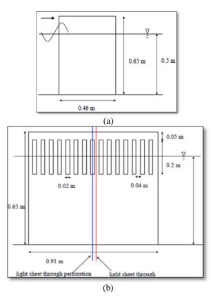
Figure 20 Sketch of perforated breakwater by Ariyarathne [5].
