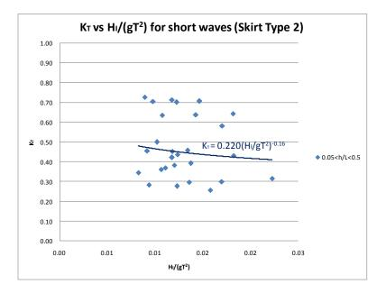
Figure 15  $K_T$  vs  $H_i/(gT^2)$  for medium depth criteria on PSB skirt type 2 investigation.
