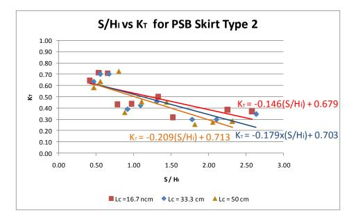
Figure 11 Transmission coefficient (K<sub>T</sub>) vs S/H<sub>i</sub> for PSB Type 2,  $T_p = 4$  s or  $T_m = 1.2$  s for Nc = 3 chambers.
