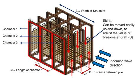
Figure 3 Some important parameters on the PSB.
