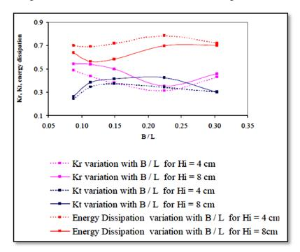
**Figure 21**  $K_T$  vs B/L,  $K_r$  vs B/L, and energy dissipation for the perforated breakwater, by Ariyarathne [5].
