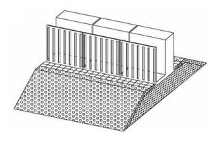
Figure 1 Perforated breakwater (introduced by Jarlan [1]).
