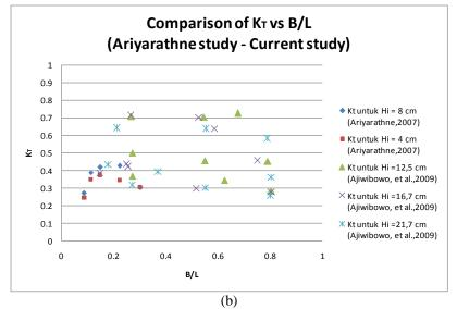
**Figure 22** Comparison for  $K_T$  vs B/L between Ariyarathne and current investigation, for: a) Skirt Type 1, b) Skirt Type 2.
