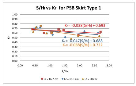
Figure 10 Transmission coefficient ( $K_T$ ) vs S/H<sub>i</sub> for PSB Type 1,  $T_p = 4$  s or  $T_m = 1.2$  s for Nc = 3 chambers.
