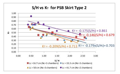
**Figure 12** Transmission coefficient ( $K_T$ ) vs S/H<sub>i</sub> for PSB Type 2,  $T_p = 4$  s or  $T_m = 1.2$  s for Nc = 3 chambers and Nc = 2 chambers.
