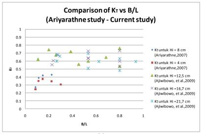
Plot for transmission coefficient  $(K_T)$  is retrieved from Figure 21 and compared to current study (presented in Figure 22).
