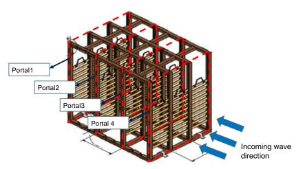
Figure 4 Definition of portal parameter on the PSB.
