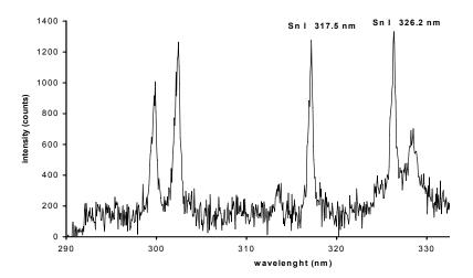
**Figure 10** The spectrum of Sn observed when a third harmonic Nd-YAG laser is focused in He gas containing ablated vapor from a solder target.
