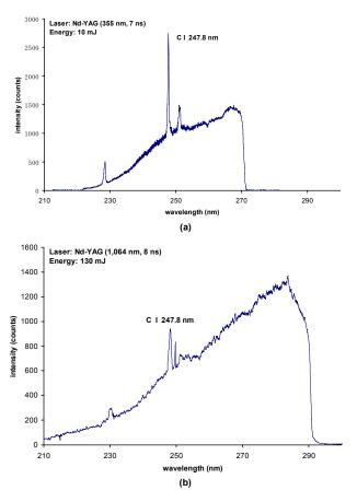
**Figure 2** Time integrated emission spectrum of C I 247.8 nm obtained for ethanol vapor. Data in (a) were obtained by third harmonic Nd-YAG laser of 10 mJ; and in (b) were obtained by fundamental Nd-YAG laser of 130 mJ. Both data were obtained in clean air containing ethanol vapor as impurity gas.
