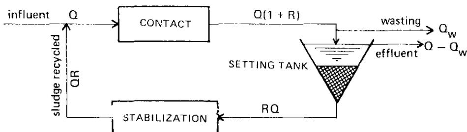
Figure 1. Flowsheet of the Contact–Stabilization Process.
