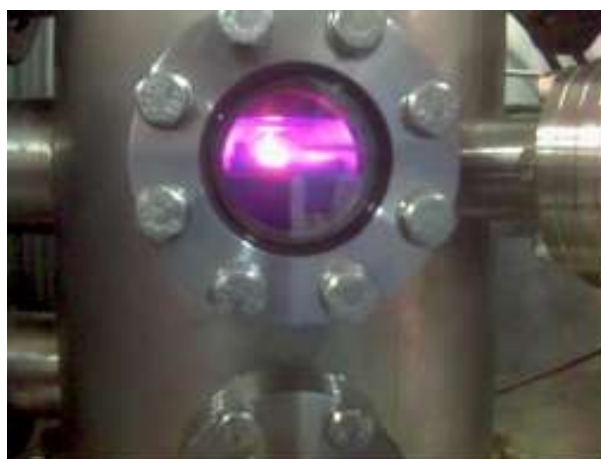
Figure 5 The plasma glow discharge of PECVD system when the hot wire filament is turned on for the CNT deposition.
