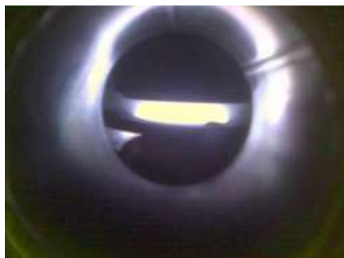
Figure 2 Glow discharge of Argon Plasma in Fe Catalyst Deposition Process.
