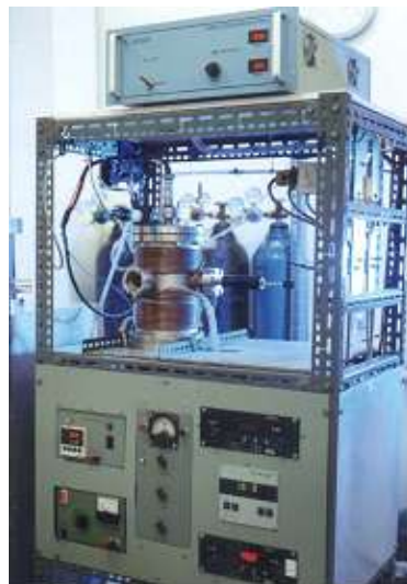
Figure 1 The existing home-made dc -UBMS system for metal catalyst deposition.
