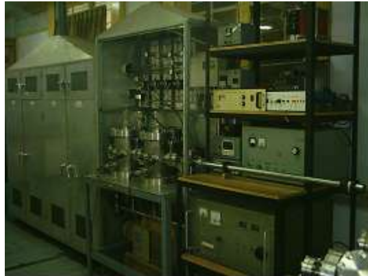
Figure 3 An existing PECVD system which is used for this research.
