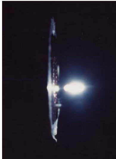
Figure 2 Photograph of the plasma generated by tight focusing 26 mJ Nd-YAG laser onto zinc sample surface under air pressure of 760 Torr.
