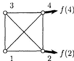
Figure 9: A  $2 \times 2$  grid with external forces in nodes 2 and 4.
