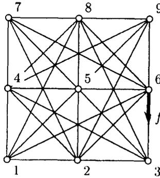
Figure 6: A 3 × 3 grid with external force in node 6.
