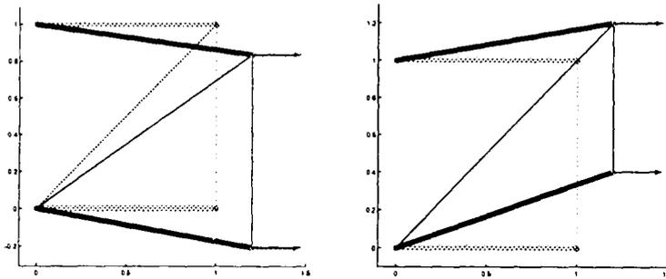
Figure 12: Multi-load truss subjected to the two separate design loads  $f_1$  (left) and  $f_2$  (right).
