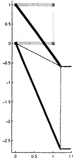
Figure 13: Instability of the multi-load truss w.r.t small occasional load.
