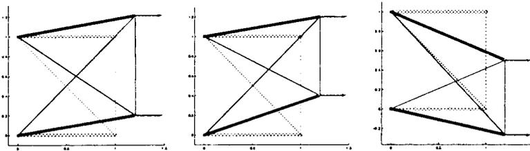
Figure 15: Multi-load truss loaded with  $f_1$  (left), with  $f_2$  (middle) and  $f_3$  (right).
