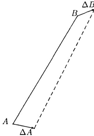
Figure 2: A bar before (solid) and after (dashed) load is applied.
