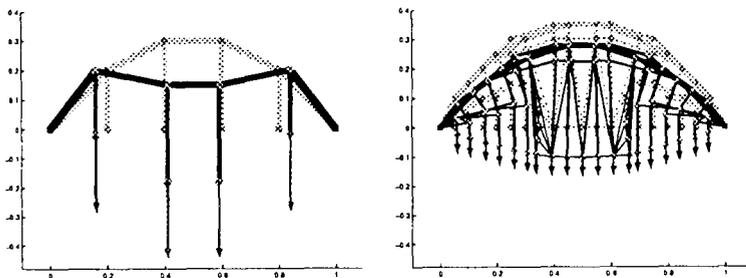
Figure 8: Trusses based on (a)  $6 \times 21$  and (b)  $21 \times 21$  grid.
