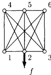
Figure 4: A  $3 \times 2$  grid with external force in node 2.
